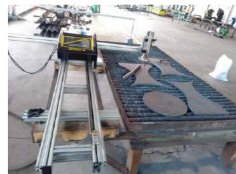
Mesin Cutting CNC Cap : 40mm x 2400mm x 4000mm
