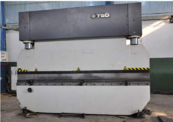
02. Banding machine with capacity 150 ton and thickness maximum 8 mm
