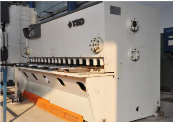
04. Shearing machine with capacity 160 ton and thickness maximum 6 mm
